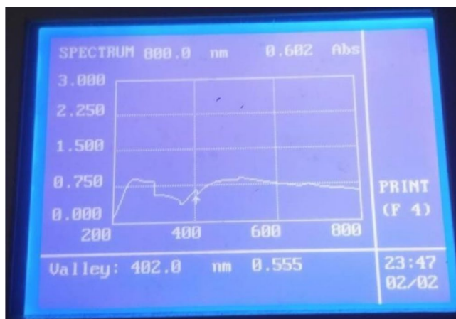
FIGURE 3 | UV-visible spectrum of aqueous solution AgNPs synthesized from M. oleifera plant.
