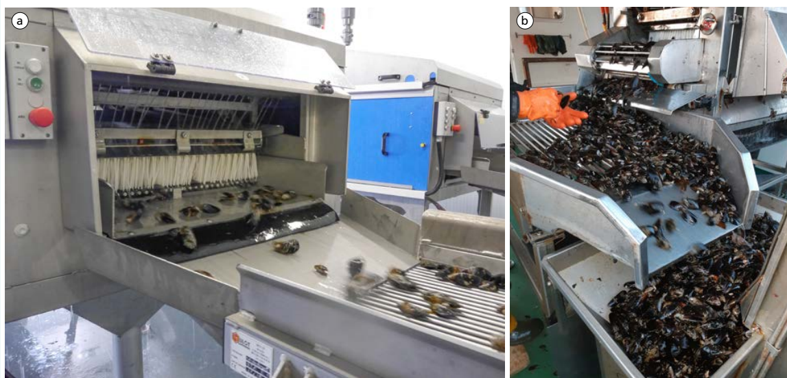
FIGURE 4.27 Examples of straight brush cleaner (a) and single grill vibrating grader (b)
