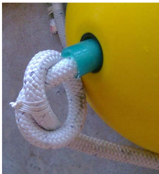
FIGURE 6.11 The knot employed on the upper side of the submersible buoy serving to secure the position of the buoy along the mooring line
