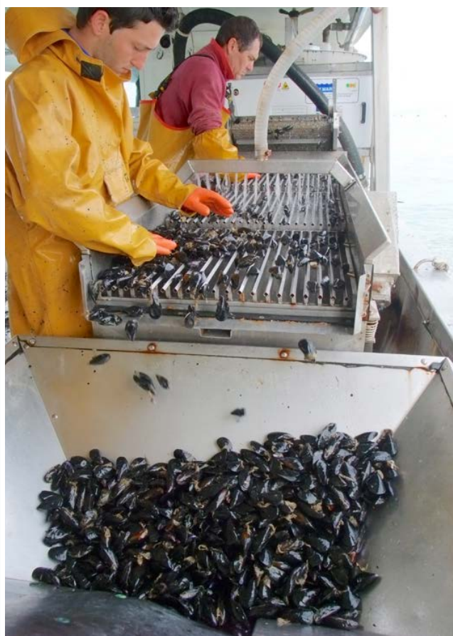
FIGURE 6.34 Declumped mussel grading on-board using a horizontal vibrating grader
