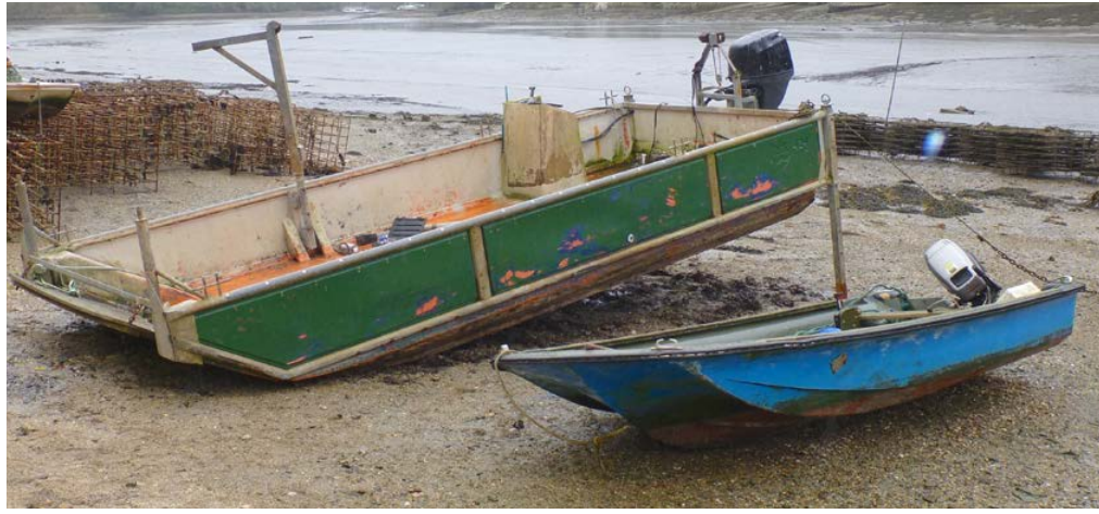
FIGURE 5.13 Example of general-purpose workboats with shallow draft and open deck space suitable for small-scale shellfish cultivation
