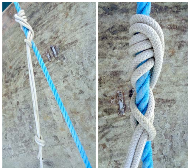
FIGURE 6.15 Temporary knot used to keep the headline in tension during positioning (views from both sides)
