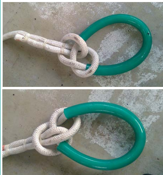
FIGURE 6.12 Extremity of the mooring line where the headline will be tied (views from both sides)
