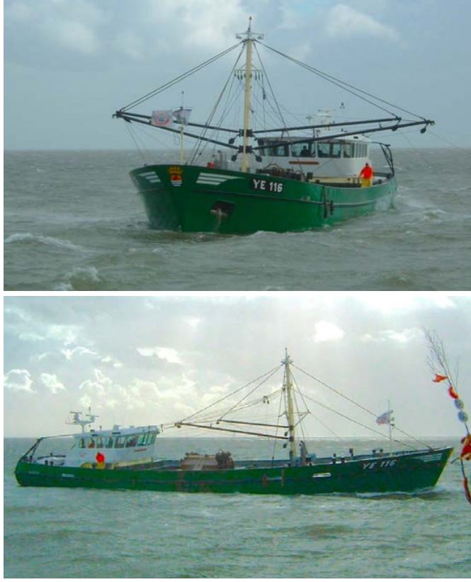
FIGURE 5.11 Mussel dredging vessel for medium- to large-scale production, fitted with derricks to deploy the dredges
