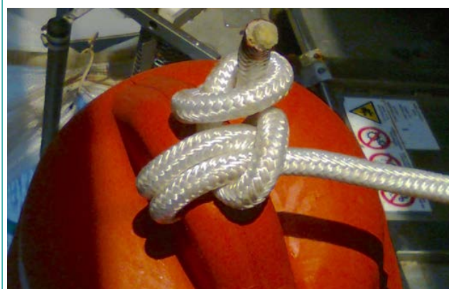
FIGURE 6.9 Knot used to secure an intermediate surface buoy Visible the security knot to prevent the rope from becoming dislodged
