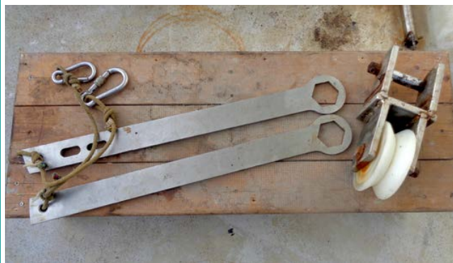
FIGURE 6.14 Wrenches and pulleys used when installing a mooring line
