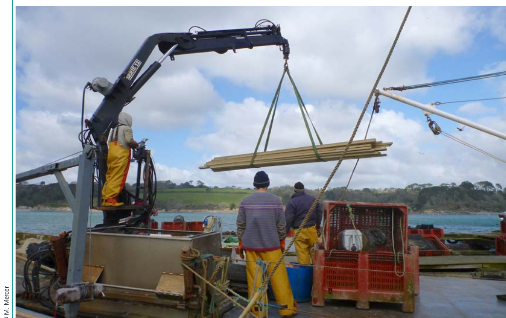
FIGURE 5.18 On-board crane used to lift farming equipment and harvested mussels
